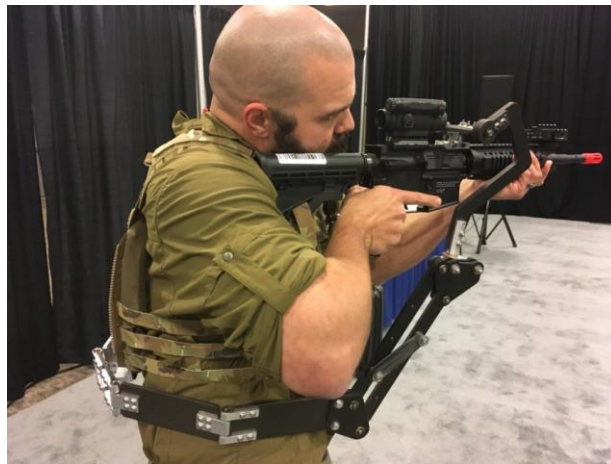
The Third Arm transfers the weight of a weapon from a soldier's arms to his torso.
